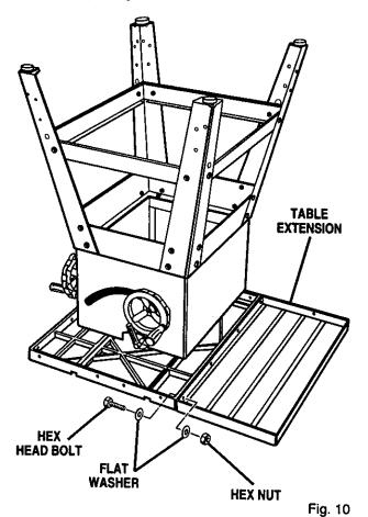
Get help to stand saw assembly upright using the center saw table. Do not grasp saw by extensions.
