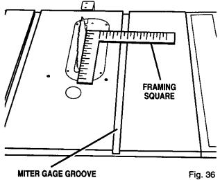
If the distances measured are different, adjust the mechanism underneath the saw.
