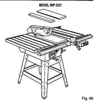
Place the work firmly against the rip fence and feed the work into the blade.
