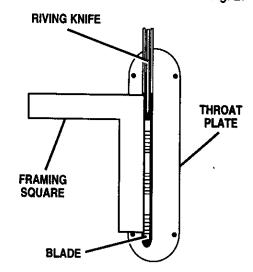
TOP VIEW OF SAW WITH RIVING KNIFE SHOWN CENTERED OVER BLADE
