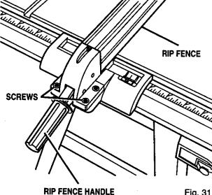
Note: To insure proper self alignment when positioning rip fence, push sides of scale indicator housing against front rail before locking rip fence handle.
